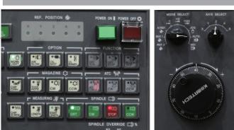
Rotary switch and On/Off buttons are added on each function for operator's convenience and common buttons are user friendly located for easy to operate and access.
