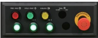
CL/UNCL, START, FEED HOLD, SINGLE BLOCK and EMERGENCY STOP buttons are separately configured on the SWITCH PANEL, ensuring ease of operation.
